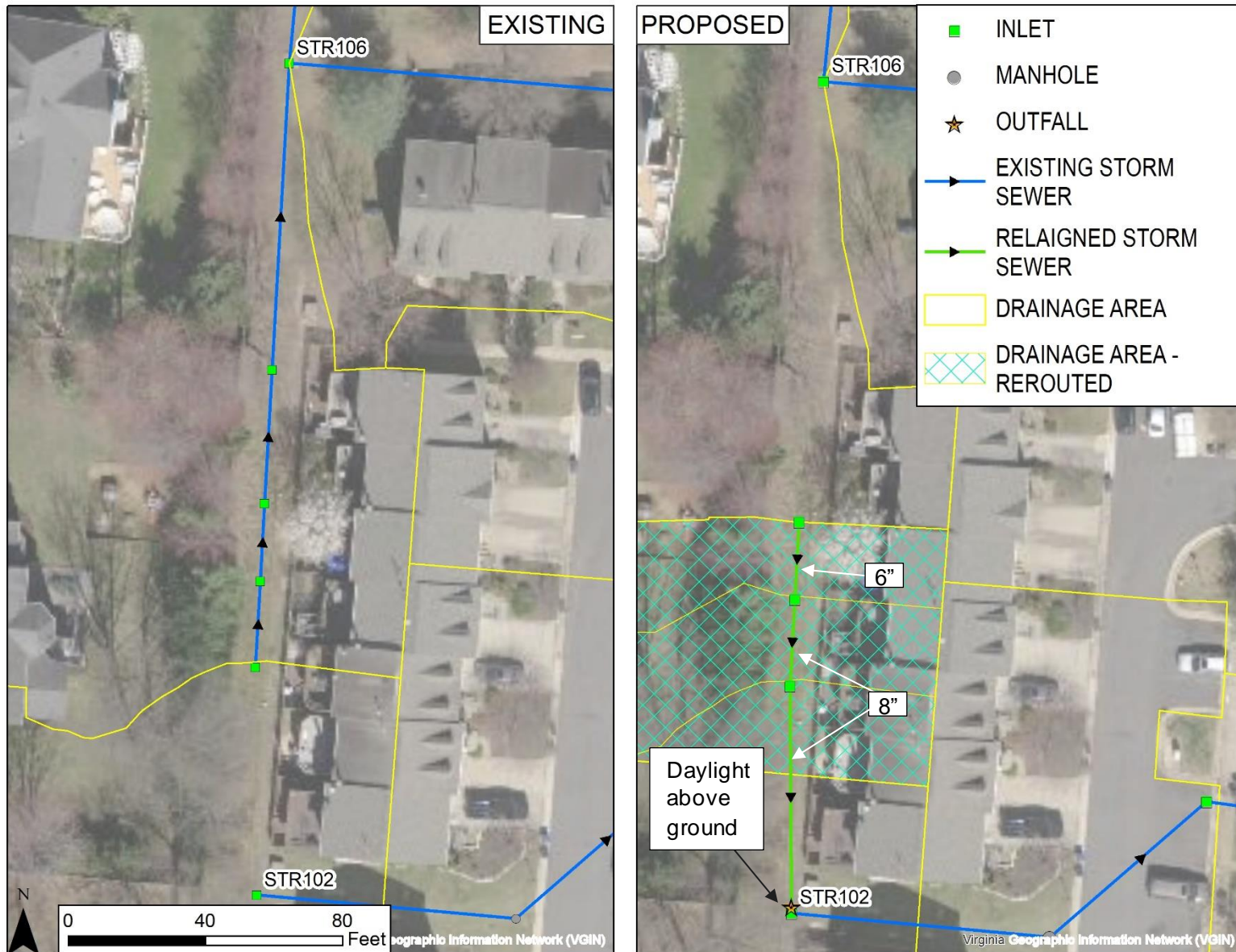
Figure 4: Proposed Storm Sewer Improvements
